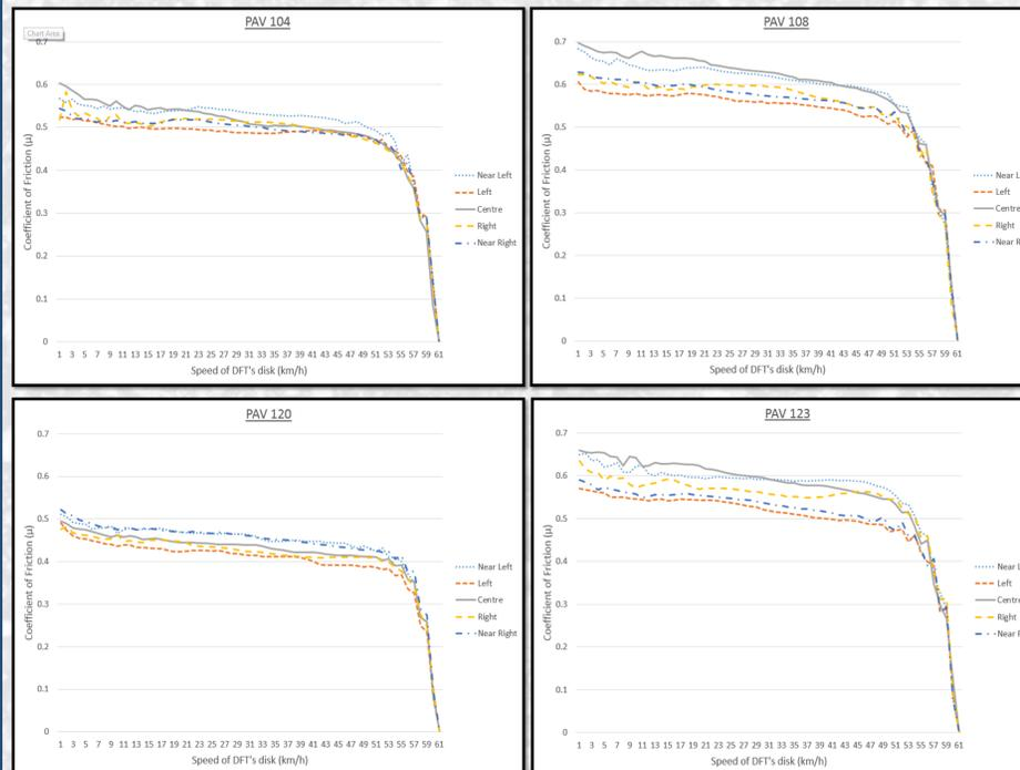
Each dataset in the table below presents the average of three test results at each location. The three DFT test results are calculated at 20 km/h, 40 km/h and the average slip speed within this speed range.
